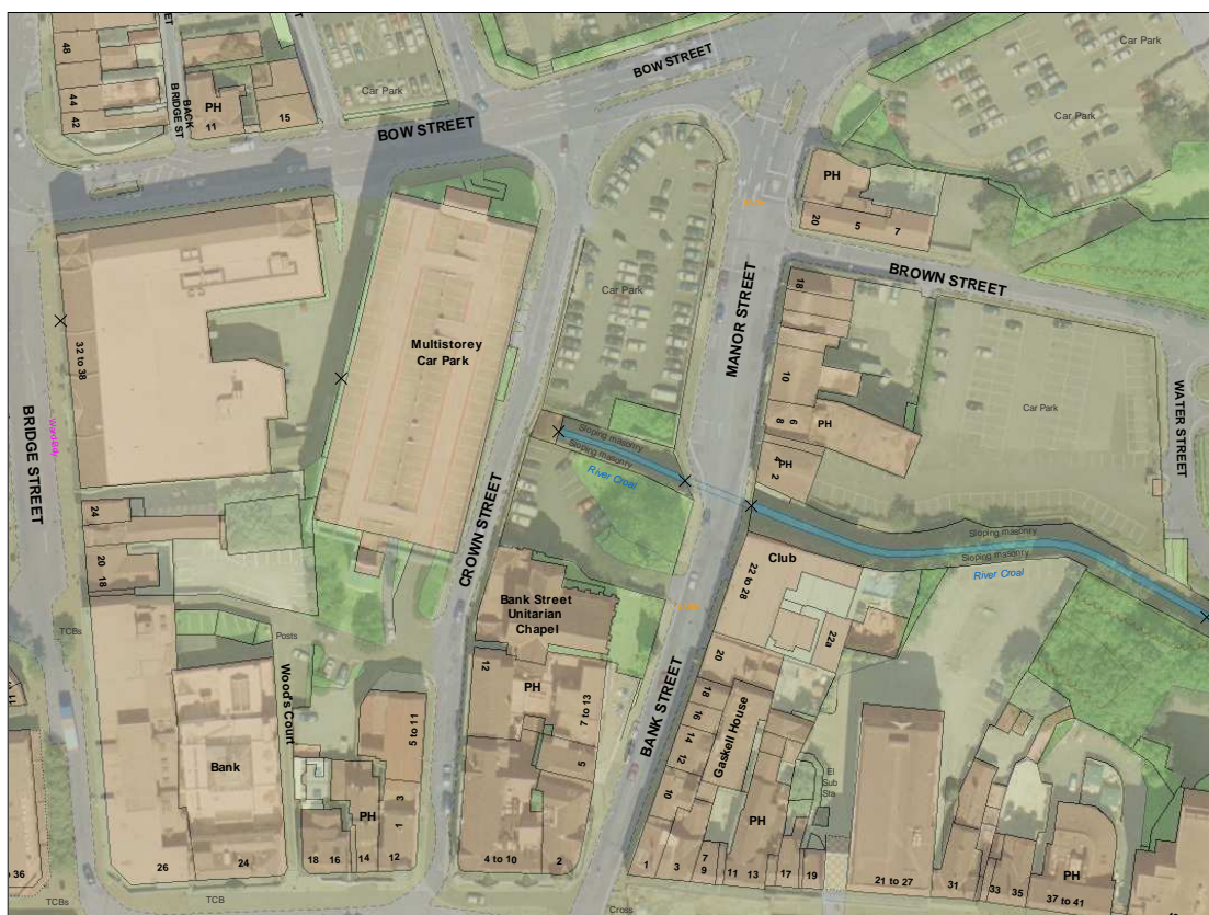
Figure 6-3: Map showing reach between Crown Street and Manor Street/Bank Street planned to be culverted as part of the Town Centre Development
