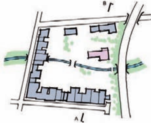
Schematic drawing of river valley site showing typical features: river corridor, outward facing street frontage on two sides, weaker edges elsewhere. Cleared internal area, mainly used for surface car parking, with surviving industrial buildings, some of historic interest. (See overleaf for cross sections)
